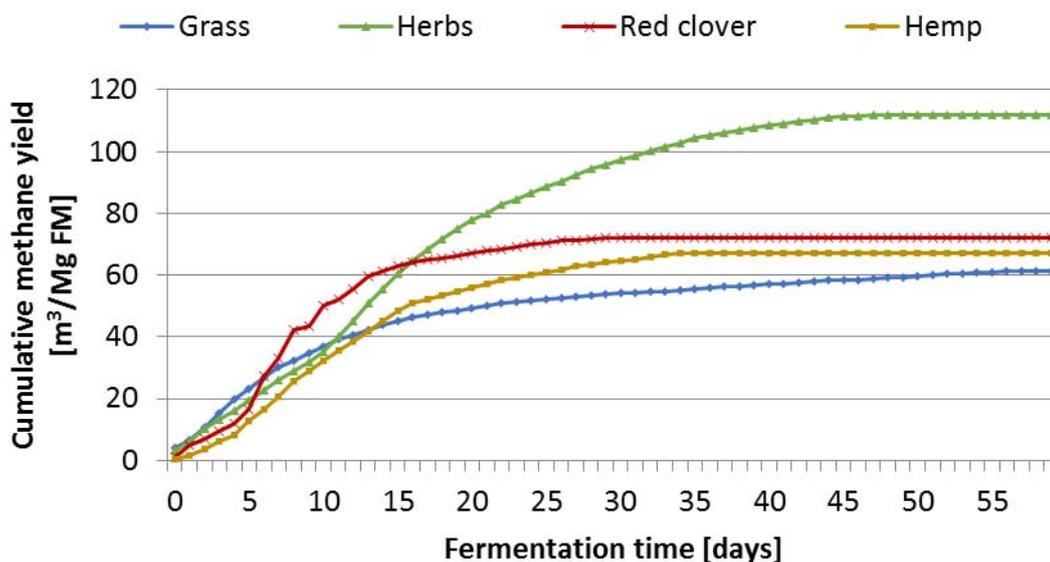
Fig. 2. Cumulative methane production [m<sup>3</sup>/Mg FM]
