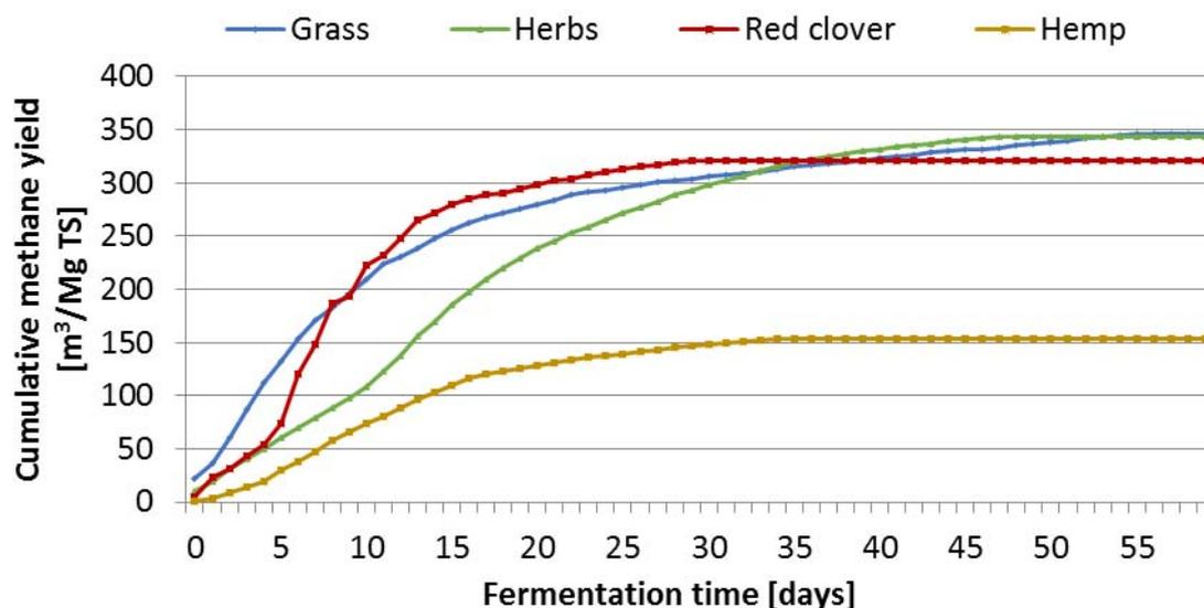
Fig. 3. Cumulative methane production [m<sup>3</sup>/Mg TS]
