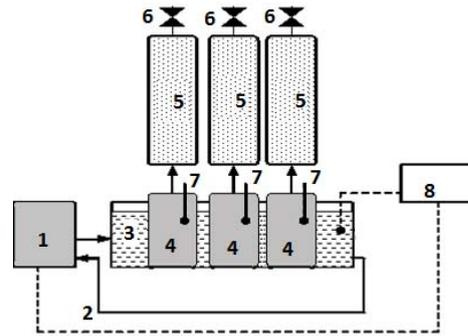
Fig. 1. Scheme of biofermentor for biogas production research (3-chamber section): 1. Water heater with temperature regulator, 2. Insulated conductors of calefaction liquid, 3. Water coat with temp. 35-42°C, 4. Biofermentor with charge capacity 2 dm<sup>3</sup>, 5. Biogas reservoir, 6. Cutting off valves, 7. Sampling tubes, 8. Recording central station
