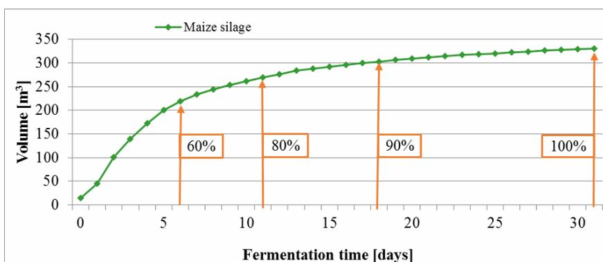
Fig. 3. Scheme of biomethane cumulative production for fermentation of maize silage
